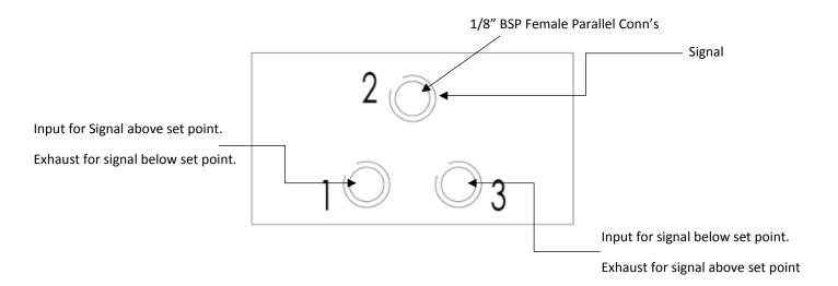
Air Supply required between 2-8 bar at 25µm filter should be fitted in the supply time.
