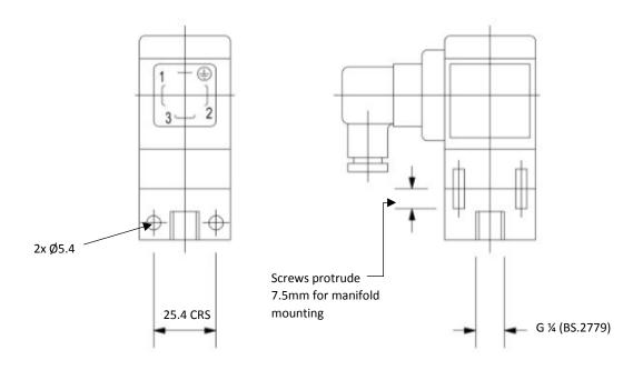
Use Terminals 1 and 2 (or C or NC) for closed circuit below operating pressure. Use terminals 1 and 3 (OR C AND NO) for closed circuit and above operating pressure.
